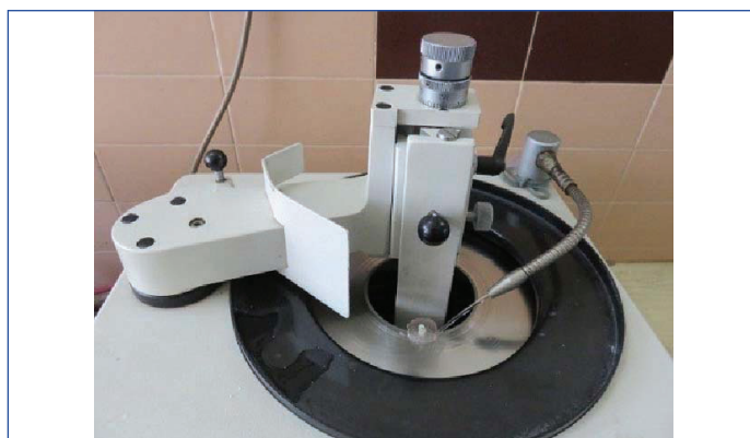
[Table/Fig-1]: Hard tissue microtome used for sectioning under water coolant with sawing action.
